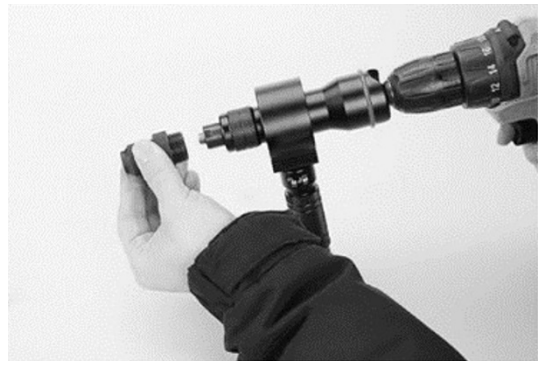
4. Install blind rivet sleeve
